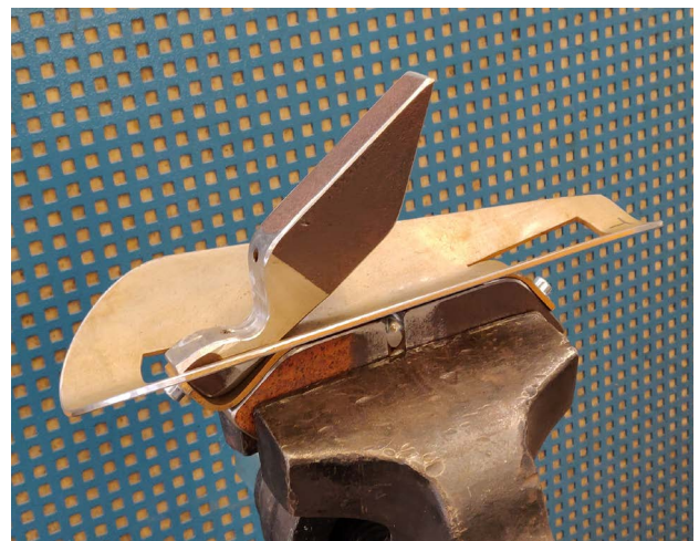
[fig.41.] special jig to bend the attachment ears
